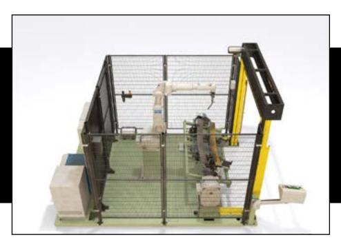
Some hazards persist even when the power is off. For example, some machines continue to move due to inertia for a short time after power is cut. And any robot fitted with a dangerous end-of-arm-tool, such as a hot welding torch or a blade, is hazardous even when still.
